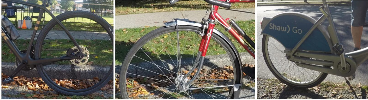
Figure 14 - Brake Classification Types (Disc, Rim, Drum)
