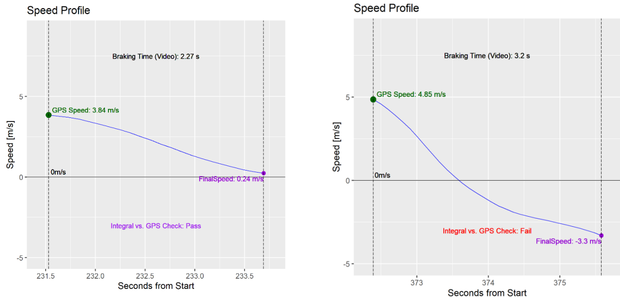
Figure 21 - Passing and Failing Speed Profiles Determined from Integrating Acceleration Data
