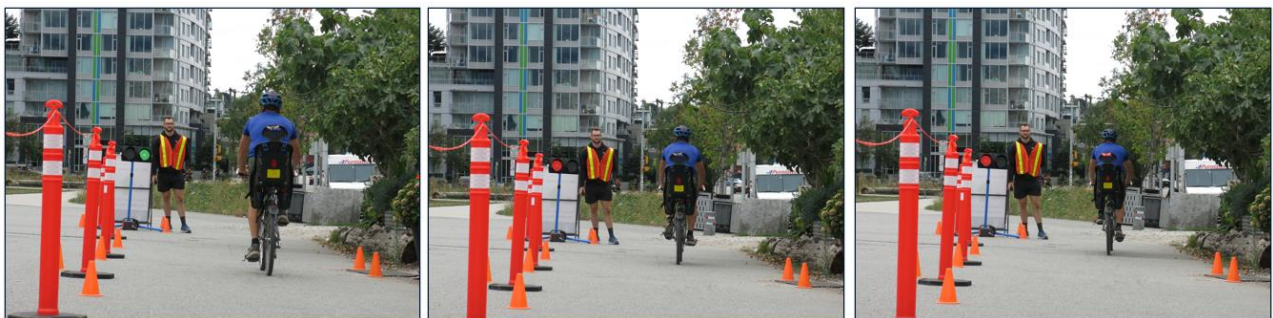
Figure 16 - Participant Riding Towards Green Light (left), Presence of Expected Stimulus, t_2 – Red Light On (middle) and Time of Brake Light Illumination, t_4 (right)
