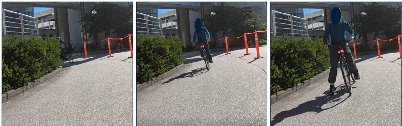
Figure 15 - Presence of Unexpected Stimulus, t_1 (left), Time of Brake Light Illumination, t_4 (middle), and Moment of Full Stop, t_5 (right)
